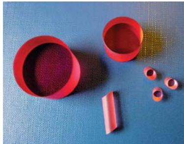
Al<sub>2</sub>O<sub>3</sub>:Ti<sup>3+</sup> indefinitely long stability and useful lifetime added to the lasing over entire band of 660–1050 nm challenge “dirty” dyes in variety of applications. Medical laser systems, lidars, laser spectroscopy, direct femtosecond pulse generation by Kerr-type mode-locking – there are few of existing and potential applications.
